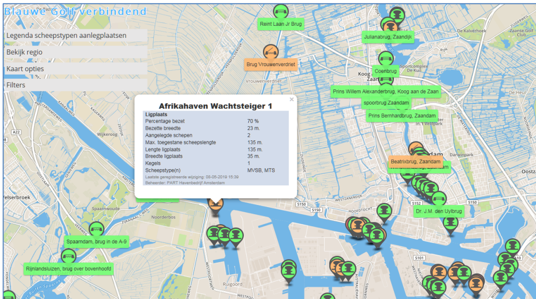
Figure 24 Data on a selected mooring place (in figure “Afrikahaven Wachtsteiger 1” in the port of Amsterdam), and other available data on the berth place or a bridge
